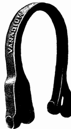
Type "J" Vanadium Steel Locomotive Transmission Bar, Bent Cold
