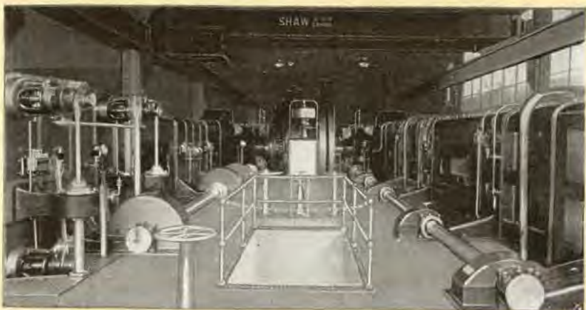
Cylinders of 6,000 H. P. Gas-Steam Engine
