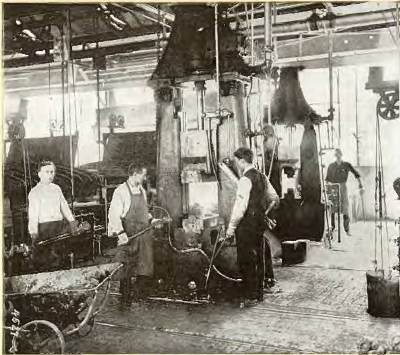
Restriking or Straightening Crankshafts on Steam Hammers
