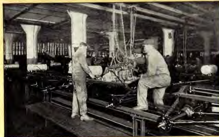
Installing Motor on Final Assembly Line
