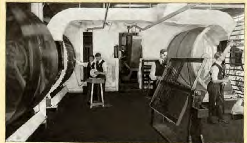
The Drying Room. Here the Film is Wound on Drums, the Air in the Room is Scientifically Washed and Tempered
