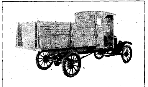
This position illustrates the Grain Body. (Inside dimensions.) Length 9 feet 9½ inches, width 3 feet 7½ inches, depth 2 feet, 5 inches. Capacity 60 bushels of wheat or other loose in proportion.
