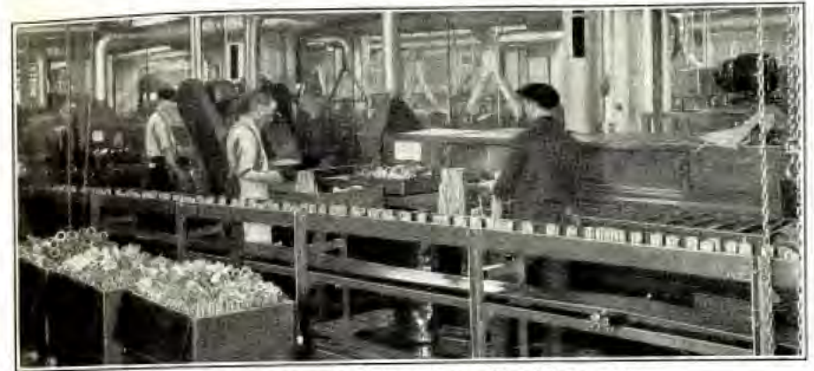
Bearings Conveyed Away After Final Inspection
