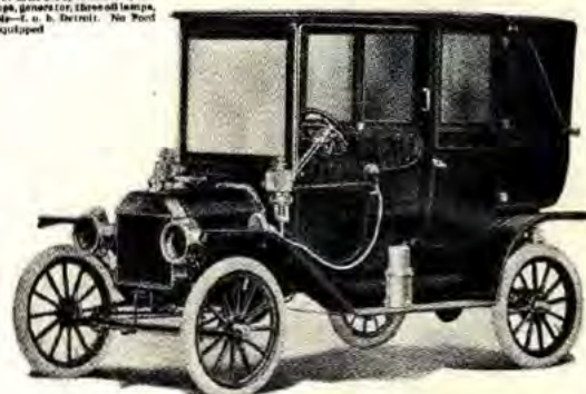
Ford Model T Four-Door Town Car (Front doors are detachable) 3-Passenger—4-Cylinder—20 Horsepower Car. Price $1400 includes speedometer, two 4-inch gas lamps, generator, three oil lamps, horn and radio—f.o.b. Detroit. No Ford Cars sold un-equipped
