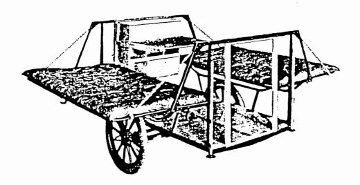
HE illustration above shows the complete Trailer before the tent covering has been attached, giving an idea of the substantial construction of the steel frame, the convenient kitchenette with inside dropleaf table and the wide comfortable mattresses which are amply supported by strong, sagless springs. This view also shows the large amount of space that is provided for baggage after the Trailer is closed.
