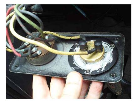
The white goo is silicon seal holding the 26-27 ammeter to the bezel ring. Disconnect the wires from the old ammeter.
