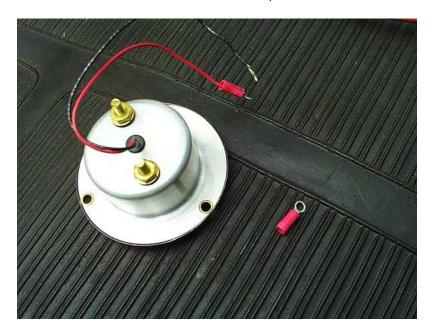
Connect the red LED wire to the tail light connector.
