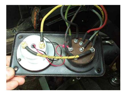
Now, connect the black ground wire to one of the ammeter screws.
