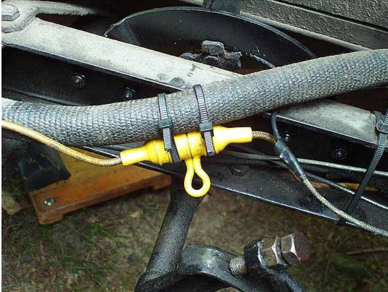
Connect the yellow power wire back up to the starter switch. Make sure all the wires are tucked in and connect up the battery.
