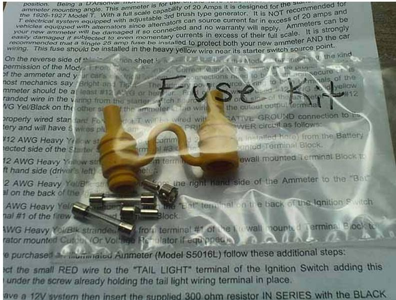
John said to put it as close to the power source as possible, cut the yellow power wire near where it connects at the starter switch, and solder the connections. He also asked if I could handle a solder gun.
