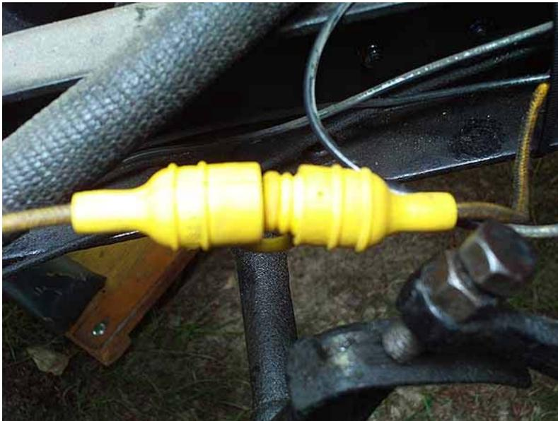
Put a couple zip ties around the housing and affix it to the cable sheath.
