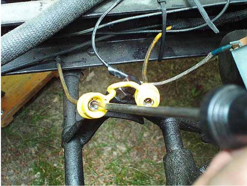
Place the fuse in and squish the waterproof housing ends together.
