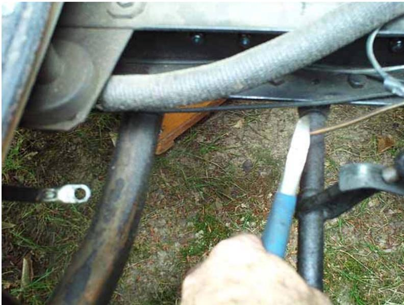
Take the short end of the power wire, twist and push it through one side of the fuse housing.
