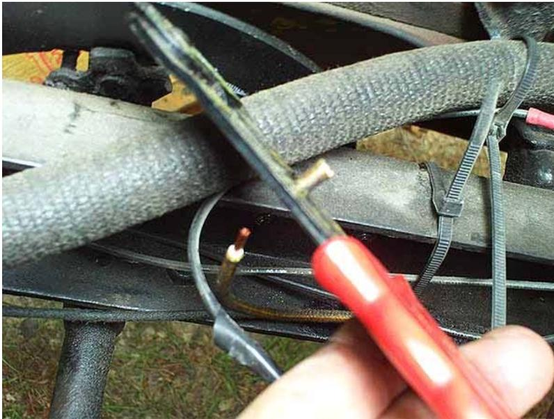
Fit one fuse connector over the wire, crimp it with the stripper, and then solder the connector on.
