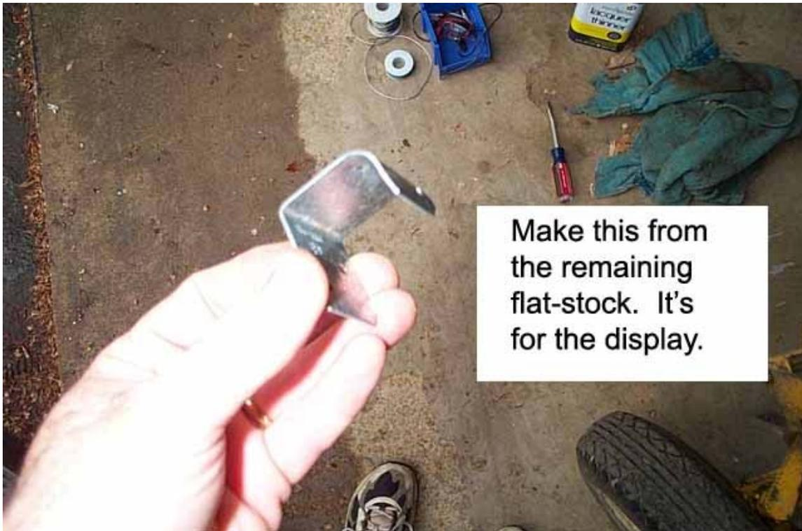
*Figure 9 – Computer Display Bracket*
