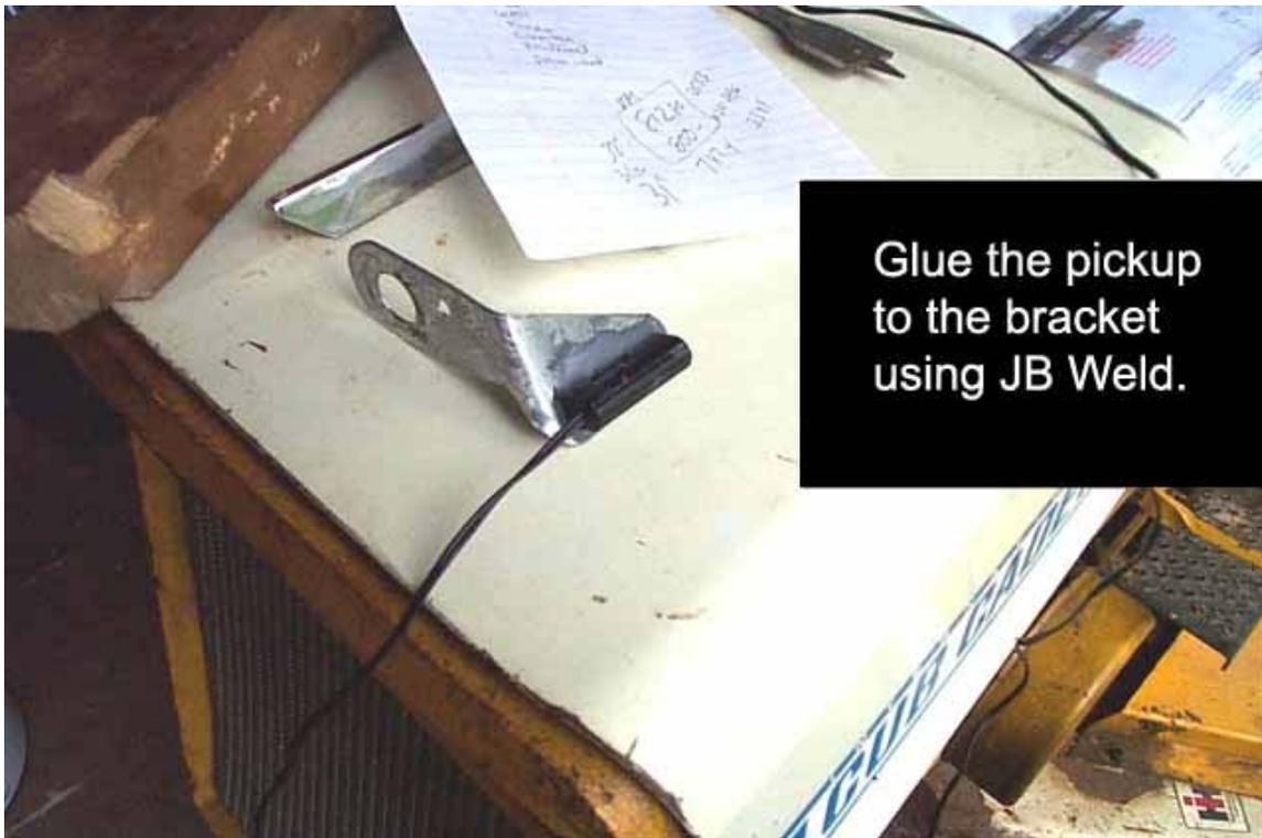
*Figure 6 – Gluing the Pickup to the Bracket*
