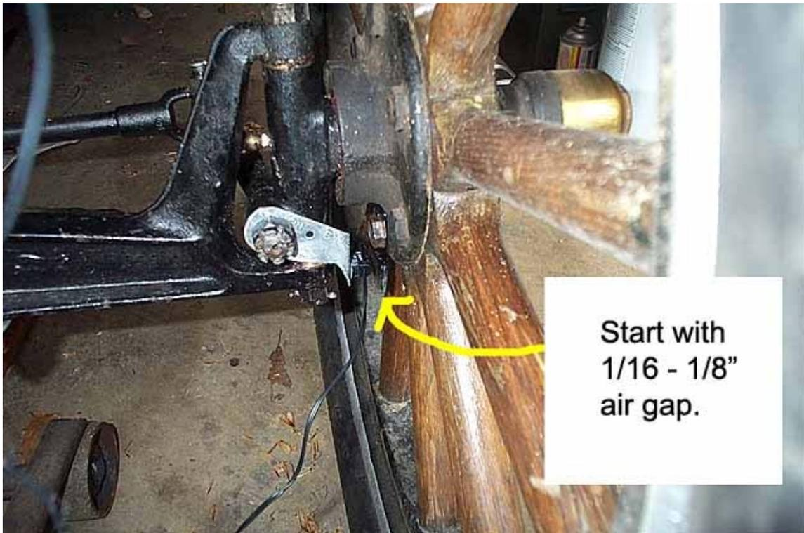
*Figure 7 – Adjusting Air Gap on Pickup and Magnet*
