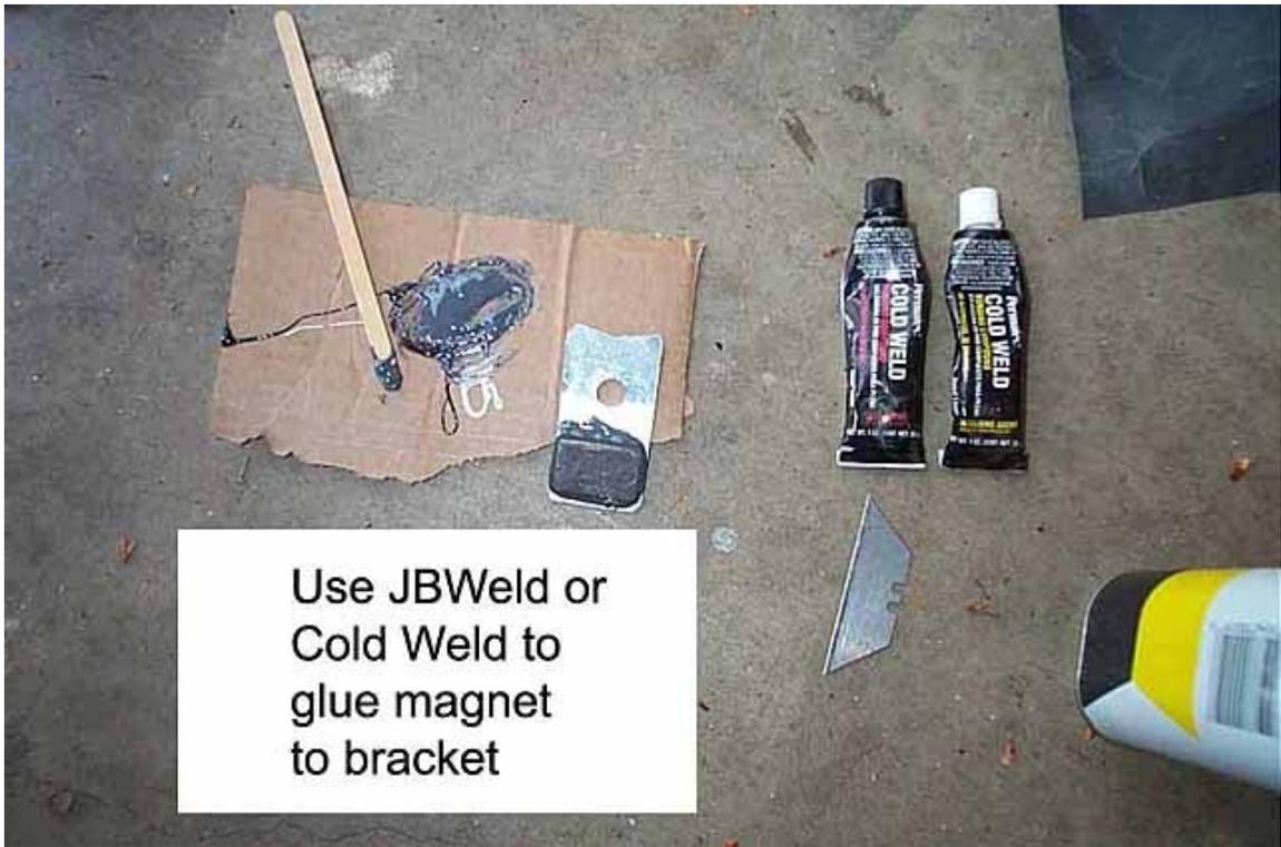
Figure 2 – Epoxy Magnet to Bracket
