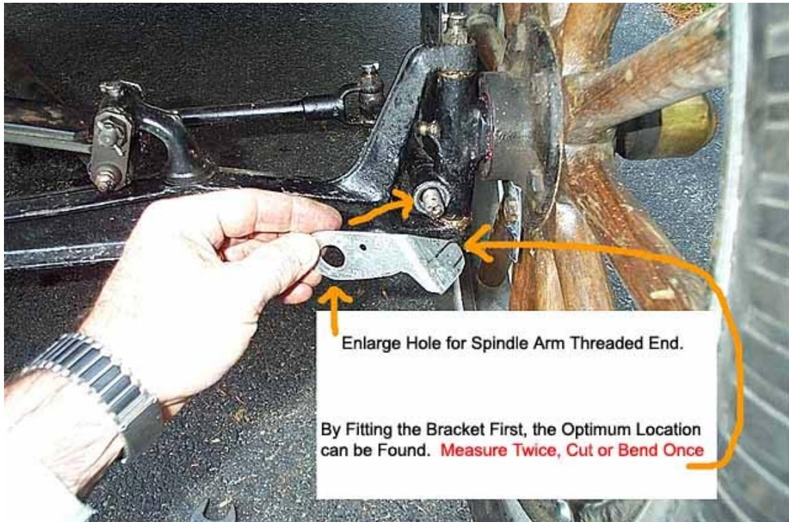
Figure 4 – Pickup Bracket
