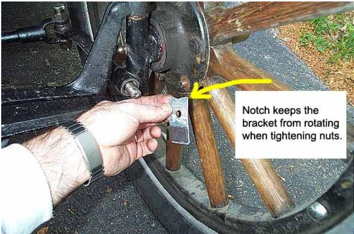
Figure 3 – Attaching Finished Bracket to Front Hub
