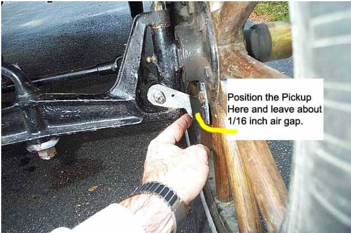
*Figure 5 – fitting the Pickup Bracket*
