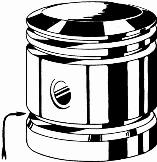
Oil pocket by bevel 3/64 " deep cut on 20^\circ angle. Fig. 33
