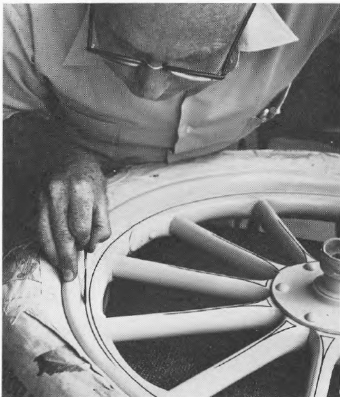
Having completed the first radial line, Mr. Clarke now starts the second radial line.
