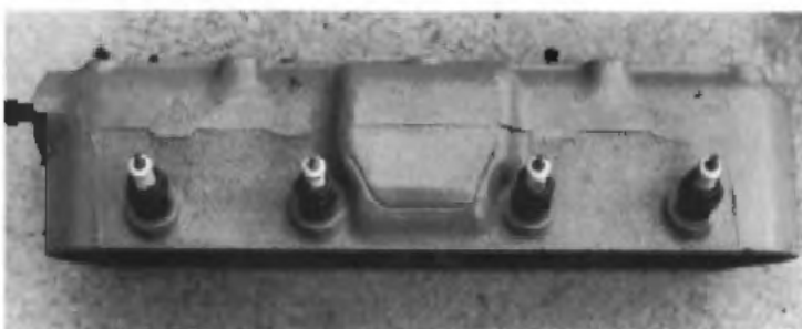
The Model 30 has a single set of 1/2-inch pipe thread spark plugs on the left side.
