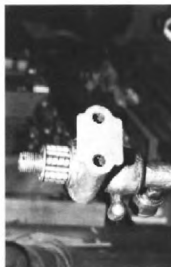
The roller bearing rocker arm used on some Model 31, B, BB and BB-R RAJO heads.
