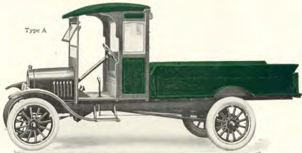
Open Express Body with Cab For the Ford Ton Truck Chassis
