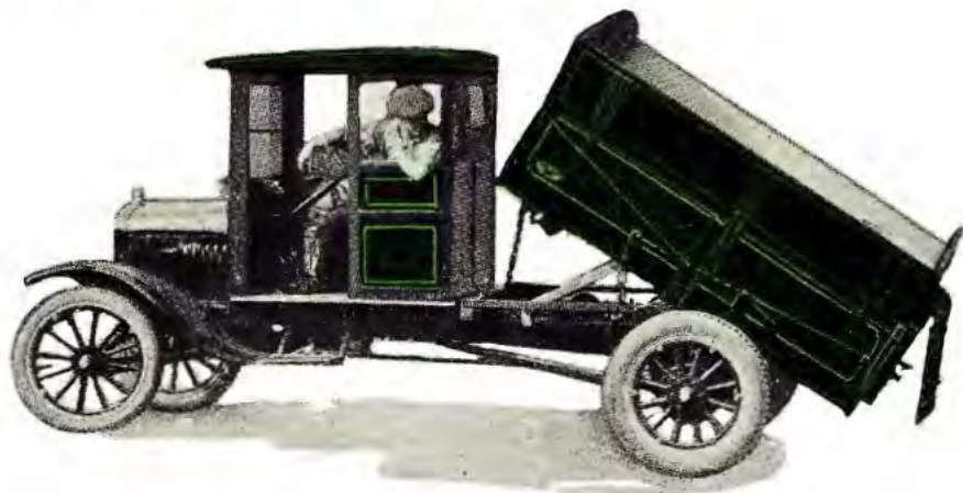
A 3 Cu. Yd. Dump Body with Drop Sides
