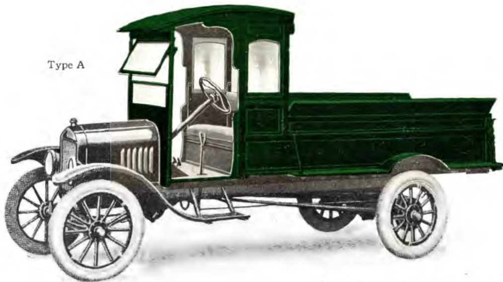
Cab Top Express Body For the Ford Ton Truck Chassis SPECIFICATIONS
