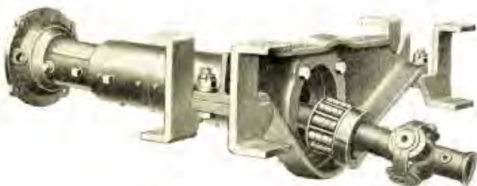
Olson Extension Shaft with Housing, Showing Steel Cross Member, Brackets, Standard Ford Universal Joint and Roller Bearing
