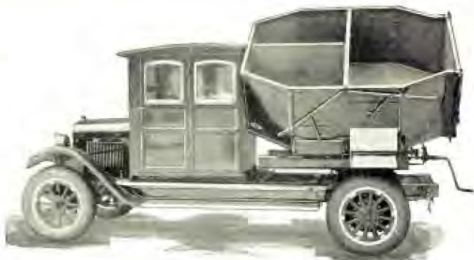
Model No. 99—Two Ton Coal Body Dumps either to right or left No Backing Up
