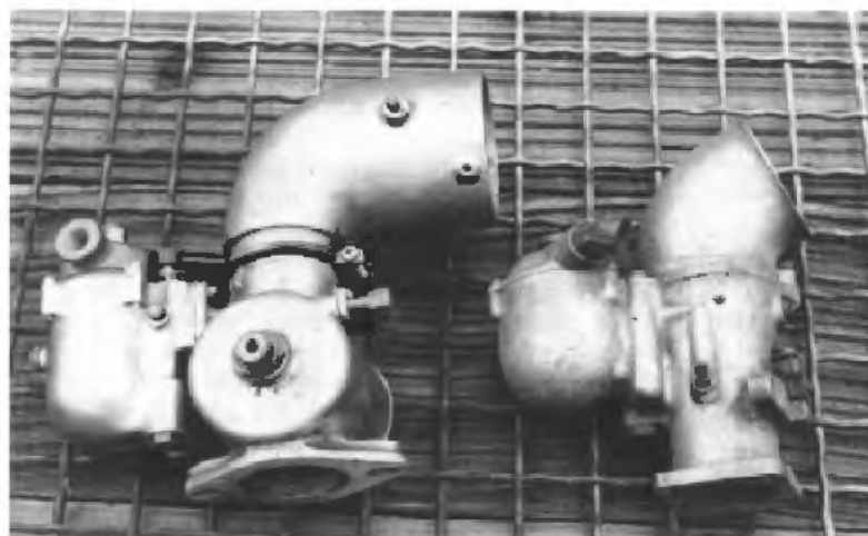
Non-standard Winfield carburetors. The left appears to be a combination of M and S features with the barrel throttle; the right one has the Model S throttle but with an integral float bowl. These appear to both be downdraft, no doubt for race cars.
