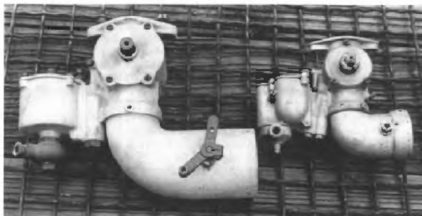
Left. An early large Winfield of non-standard design, perhaps used on a race car. Right is the second type, the Model M. All of the Model M were apparently updraft.
